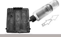
S-I-o-w-I-y and gently squeeze the ink refill bottle to force ink into the cartridge. This must be done with very little pressure, pulling the needle upward as you go. Each chamber takes approximately 5ml of ink.
